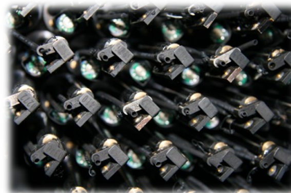
Figure 2 shows the fiber positioning units
