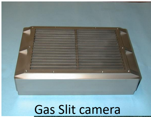
Principle of the MAXI Slit Camera; it consists of slit & slat collimators and a one-dimensional position sensitive X-ray detector.
